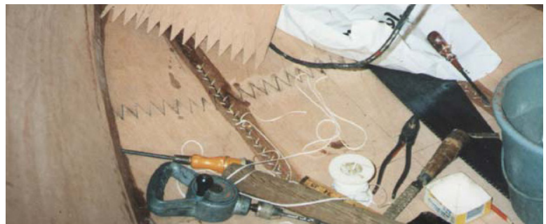
Joining the zig-zag splicing. 2nd image shows examples of splicing, stitching and the various hand tools needed.
