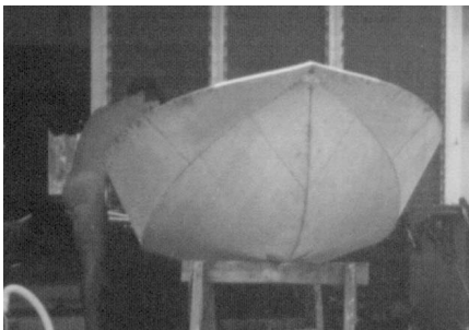
Construction showing the 'shell' of the dinghy being pulled and stitched into shape with edges butted together.
