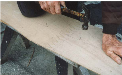
Joining the zig-zag splicing. 2nd image shows examples of splicing, stitching and the various hand tools needed.
