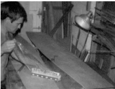
Dinghy under construction showing cut outs of panels prior to sewing together, 3rd image shows hull beginning to take shape
