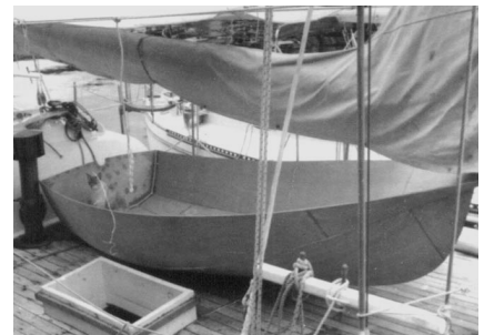
Construction showing the 'shell' of the dinghy being pulled and stitched into shape with edges butted together.
